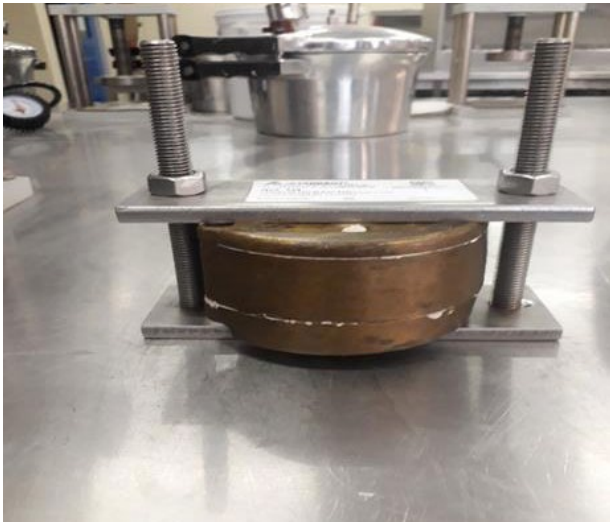
Figure 2: RS flask closure method
